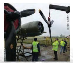
With the expert help of the DAS military vehicle wing we removed the propellor
